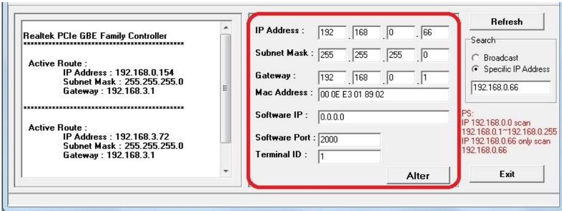
4. The showed information of MX60L2 can be revised directly in the window, the part can be modified: IP Address, Subnet Mask, Gateway, Software IP, Software Port, Terminal ID. After modification completed ( MAC Address can not modify ),click [Alter](#) then it will display the modified information, as shown:
