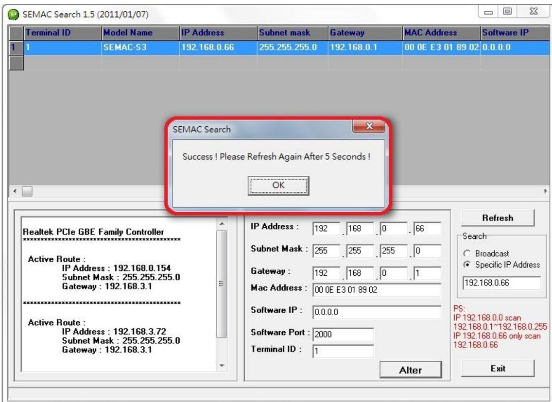
5、After modification, if want to confirm whether the modification is correct or not, click Refresh button to refresh and check information ( Fig-1 ), click Exit button to leave.(Fig-2)
